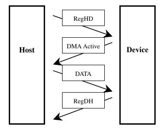
Figure 5.17 DMA data-out command protocol
